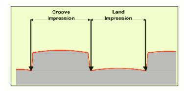
The measuring of land and groove impressions on a fired bullet can be accomplished by utilizing either the air-gap method, the LCD method or one of the stereo microscope methods. It may be necessary to measure several suitable land and groove impressions to obtain a reliable measurement. Measurements taken are recorded into iLIMS.
