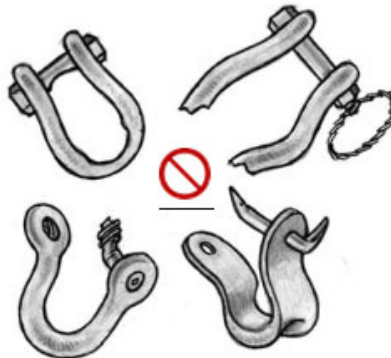
REPLACE SHACKLES THAT ARE BENT, BROKEN, OR SHOW EXCESS WEAR ON THE INNER SURFACES.
