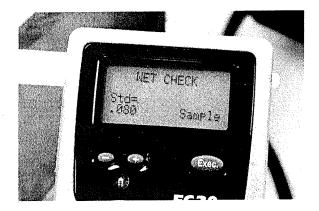
Now the display shows "Wet Check" and the target value of the standard. Use the + and – keys to adjust the value to the target of the solution you're using. This value comes from the **certificate of analysis** issued by ISP and might be slightly different from what the bottle label shows.
