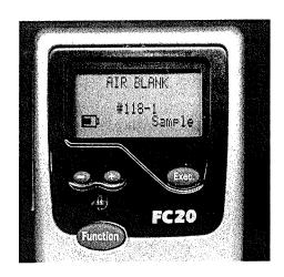
condition. To get a more accurate indication of battery condition, press Function repeatedly until the Status window appears, then press Exec./Function/Function to see the actual battery voltage. At 4.4 volts the instrument will no longer operate and the display will show "Warning Low Battery". Replace with fresh alkaline batteries.
