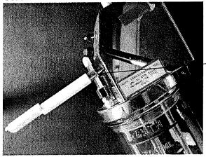
Short piece of clear tubing on "vapor out" tube of simulator.
