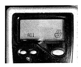
To print just calibration data, press the +/- buttons until the display reads "Cal/Cal Check" and you can print out the last calibration and calibration check data.
