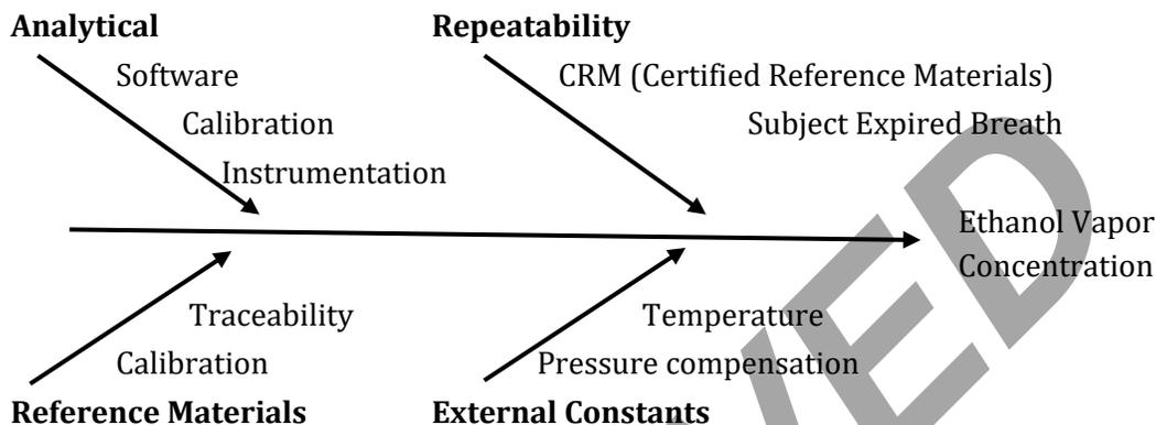
2.6.8 **Figure 1** is a cause-and-effect diagram showing the uncertainty sources incorporated into the budget for the breath alcohol reference materials. It applies to both the external standards and the instrument calibration and measurement process. There are four major components that contribute to the overall uncertainty, and they are broadly categorized as: analytical (Type B), repeatability (Type A), reference materials (Type B) and external constants (Type B).
