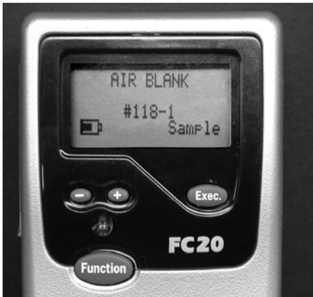
To get a more accurate indication of battery condition, press **Function** repeatedly until the **Status** window appears, then press **Exec./Function/Function** to see the actual battery voltage. At 4.4 volts the instrument will no longer operate and the display will show "Warning Low Battery". Replace with fresh alkaline batteries.
