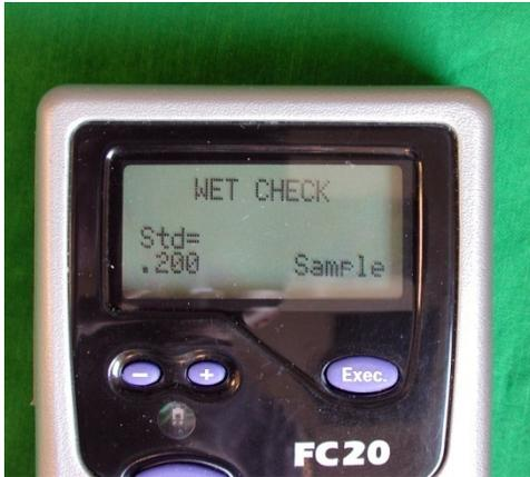
Final step: Reset the “Std=” value to the target for the 0.08 simulator solution.
