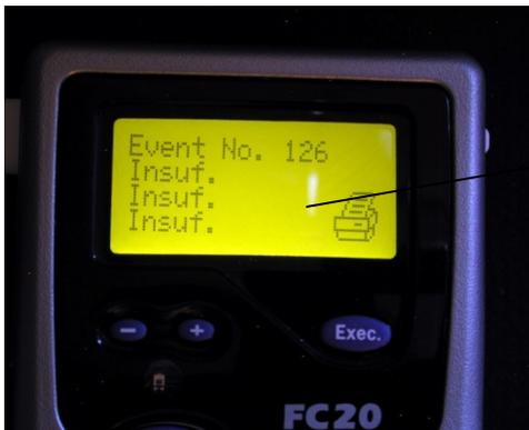
All three tests were “Insufficient”
