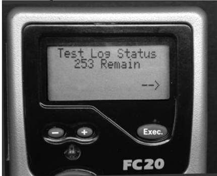
From this window, pressing **Function** takes you to the Battery Status display. Pressing **Exec.** while in the Test Log Status window takes you to this display:
