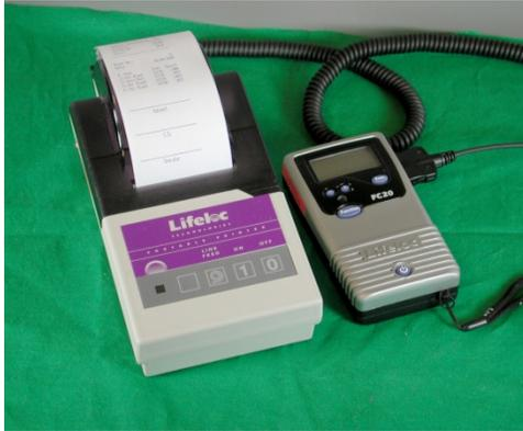
Connect the printer cable with the notches facing forward and the screws facing up. Attempting to force a connection with a printer cable in the wrong position may damage the instrument.
