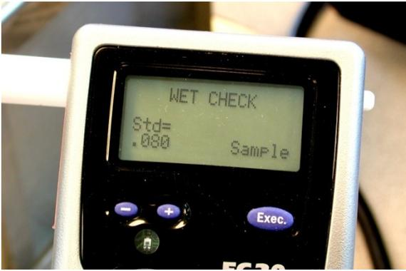
Now the display shows “Wet Check” and the target value of the standard. Use the + and – keys to adjust the value to the target of the solution you’re using, for example 0.200 or 0.080. This value comes from the **certificate of analysis** issued by ISP.
